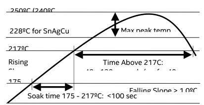
interactions that each profile adjustment makes, it can be very difficult to develop a rework profile. This is especially true if all stages of the profile are targeted for development simultaneously. A recommended approach is to break the profile down into phases, and develop the first phase first, then the second, and so on.
